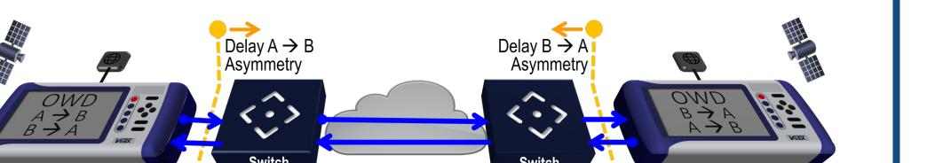
PTP assumes symmetrical data links, but longer delay in the M-S (forward) direction causes the T-SC to have negative TE, while longer S-M (reverse) delay causes positive TE.
